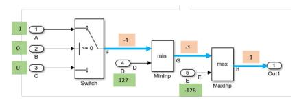
To generate test cases for enhanced MCDC, in the Configuration Parameters dialog box, on the **Design Verifier > Test Generation** pane, for **Model coverage objectives**, select Enhanced MCDC. Then perform test generation analysis. For more information, see Enhanced MCDC Coverage in Simulink Design Verifier.
